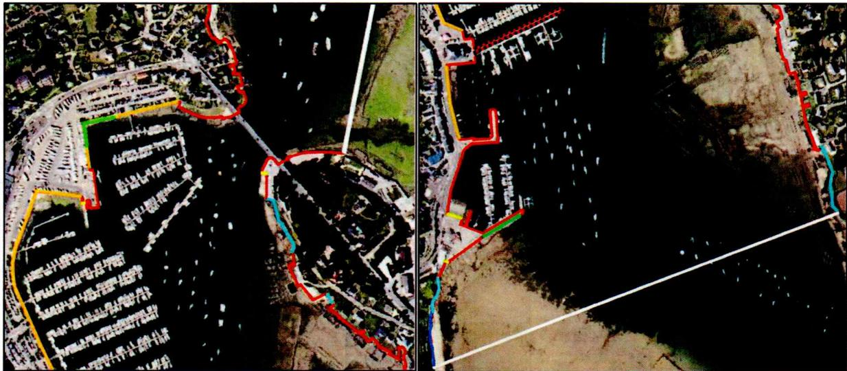
FIGURE 13 : REPRESENTATION DES COEFFICIENTS DE REFLEXION APPLIQUES AU CONTOUR – ETAT ACTUEL
