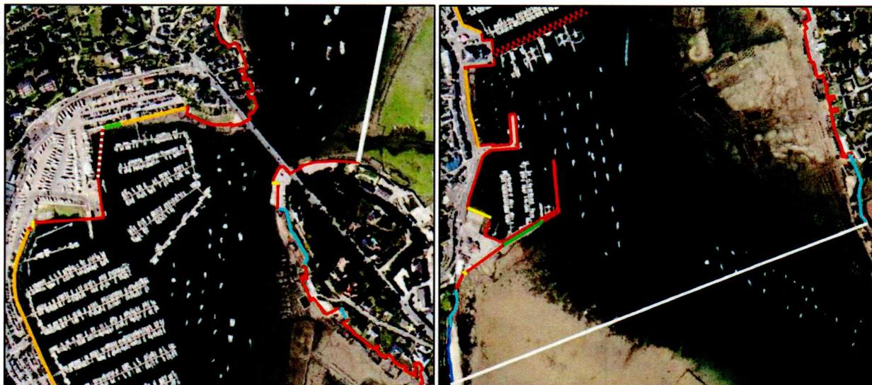
**FIGURE 14 : REPRESENTATION DES COEFFICIENTS DE REFLEXION APPLIQUES AU CONTOUR – ETAT PROJET**
